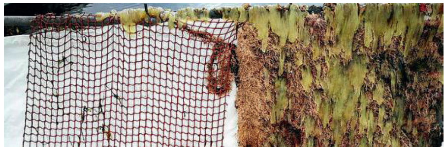
Net panels with and without antifouling impregnation. Photo: Steen-Hansen AS
